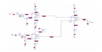
The IC's U1 and U3 get the input from the current sensor and voltage sensor respectively. They convert it to square waves which are in phase with the input waveforms. In the IC U2 the square waves corresponding to Current is subtracted from the square wave corresponding to Voltage. This gives an output signal which is a square wave whose duty cycle is inversely proportional to power factor. By measuring this duty cycle the Arduino directly gives us the Power factor.
